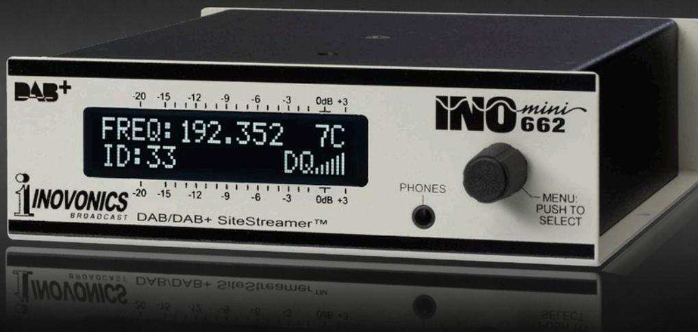
The INOmini 662 SiteStreamer™ is a Web-enabled EBU-standard DAB / DAB+ digital radio receiver for program audio and confidence monitoring. It permits the program originator to hear his broadcast and measure certain important parameters at a remote location, even where the off-air signal cannot be received. A StationRotation™ feature can be programmed to sequentially scan up to 30 station presets.
